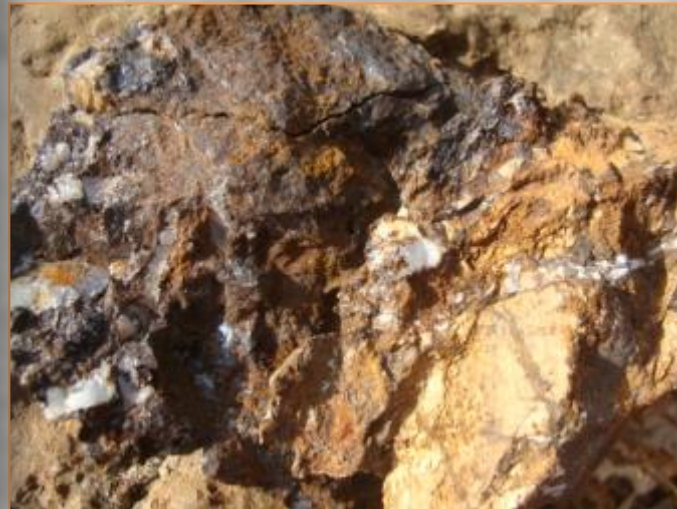
Limonitised quartz stockwork: Komto primary gold mineralisation
