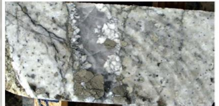
Figure 13: Albitised syenite cut by a vein with quartz, carbonate and pyrite. Core specimen TKBH-010 (photo Pollard 2008)
