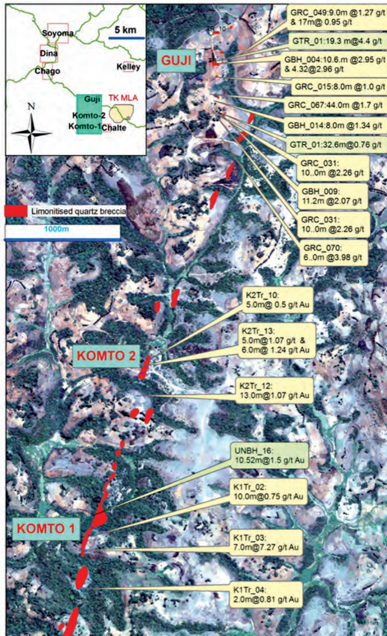
Figure 24: Best trench (and 1970 UNDP drill hole) results (2015) in the Komto 1 and 2 prospects and best drill intercepts at Guji, in the Yubdo EL. The Komto-Guji corridor is over 6km in strike and only limited drilling has tested the oxide and sulphide potential
