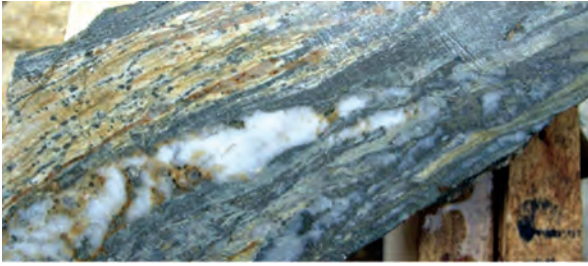
Figure 11: Quartz and pyrite in albitised syenite overprinted by a shear fabric. GKP-11. (photo Pollard, 2008)
